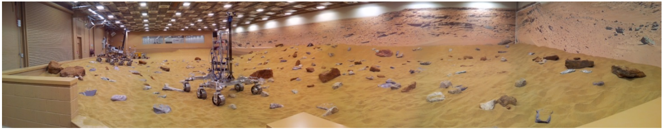
Figure 6.11.: Panoramic picture of the ASU Mars Yard with two Bridget rovers and the control room in the far side (Courtesy of Airbus).
