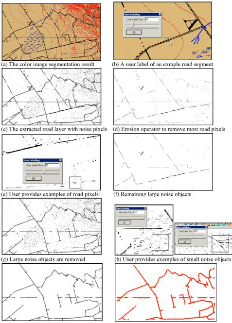
(i) Noise objects are removed Fig. 2. Road layer cleaning with minimal user labeling
