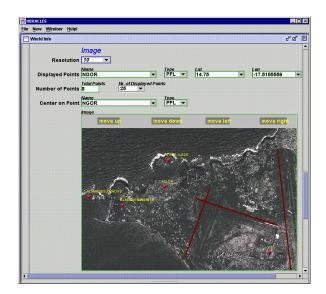
Figure 6: Satellite image of the selected airport with the vector data for the three runways
