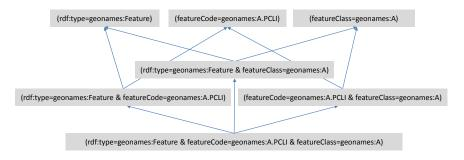
Fig. 1. Hierarchy showing how restriction classes are built
