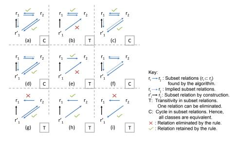
Fig. 6. Eliminating Implied Alignments
