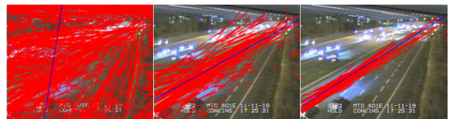
Figure 2: Segments from three clusters along a single path in the cluster hierarchy tree. (Left) root cluster. (Middle) A cluster with large variance and a large number of samples. (Right) A cluster with small variance and a large number of samples, representing a road boundary.
