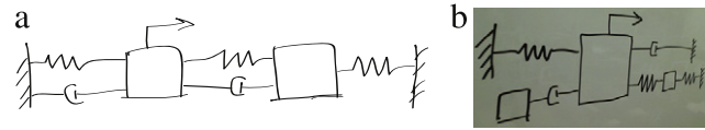
Fig. 2. Local visual variations are the major challenge for sketched symbol recognition. (a) Sketched diagram of a mechanical vibration system that exhibits high variability in drawing styles, scales, local distortions and over-tracing strokes. (b) A webcam snapshot of a rectilinear mechanical vibratory system that has undergone foreshortening due to the relative position between the webcam and the drawing board.
