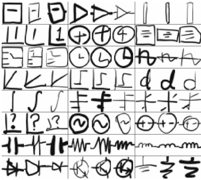
Fig. 10. Sketched symbols from the Sym24 data set, showing three examples per class. From left to right, top to bottom: scope, gain, mux, constant, sum, transfer function, clock, sine wave, step, derivative, integration, sign function, Columbus friction, random number, AC source, V source, capacitor, resistor, inductor, diode, transistor, ground.
