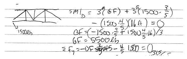
Figure 1. Example of typical student error: Internal forces (GF and DF) are not drawn on section, but appear in equilibrium equations; the solutions ultimately have sign errors.
