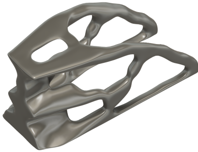
(d) Optimized topology with segmentation. c = 148 , H_{\bar{\alpha}} = 0.118
