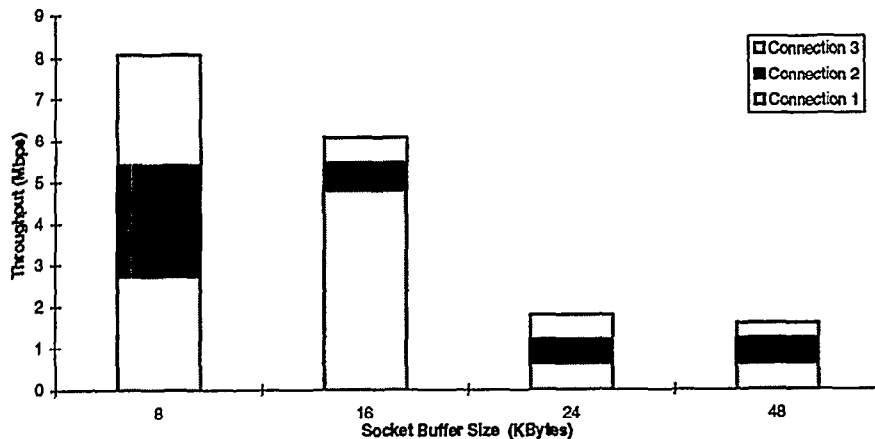
Fig. 10. Variation in throughput for different TCP socket buffer sizes when three connections simultaneously access the HFC network via a CM with a 10-kb buffer.
