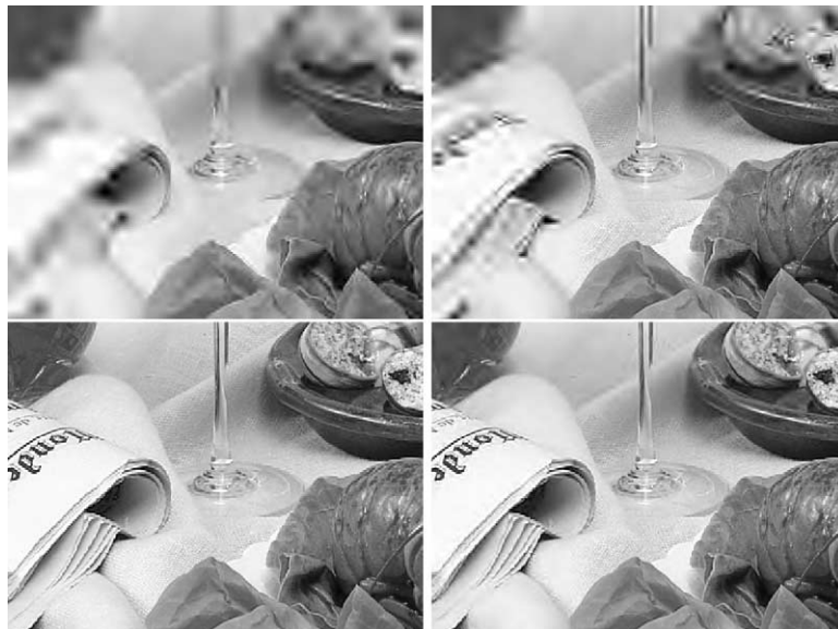
Fig. 5. Magnified portions of the “bike” image, encoded at 1.98 bpp, with a ROI, and decoded at 0.03125, 0.177, 0.5 and 1.98 bpp, in clockwise order. The ROI occupies the lower-right half of the image, approximately.
