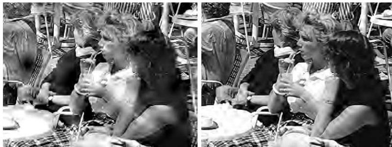
Fig. 16. Magnified portion of the “cafe” image coded with JPEG 2000 at 0.5 bpp, when transmitted over a channel with bit error rates of 10^{-4} (left) and 10^{-5} (right). The images shown are the ones with median MSE, of 200 runs.
