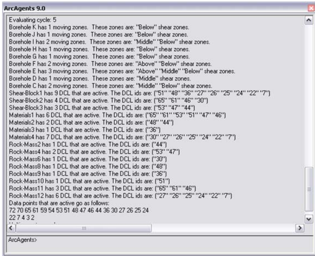
Figure 4 - The results from one cycle in the slope monitoring application
