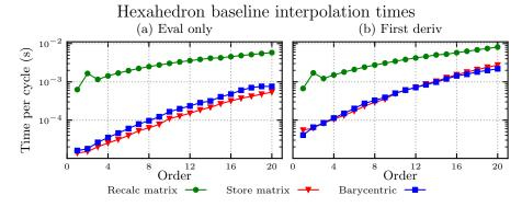
Fig. 5 Baseline interpolation timings for a hexahedron. (a) Only physical values, (b) Physical and first derivative values.
