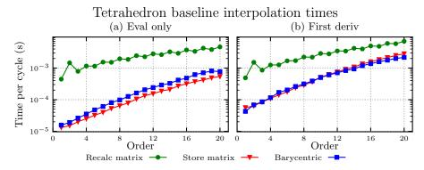
Fig. 7 Baseline interpolation timings for a tetrahedron: (a) Only physical values and (b) Physical and first-derivative values.
