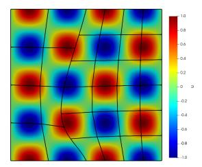
Fig. 9 The nonconformal mesh for the real world usage example with the initial projection of the u field overlaid.
