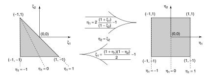
Fig. 2 Right-sided triangle to reference quadrilateral transformation.
