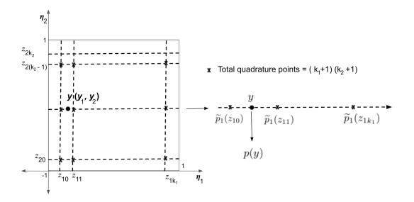
**Fig. 1** Application of univariate procedure in a dimension-by-dimension way. Evaluating  $\tilde{p}$  as an intermediate quantity and using that quantity to evaluate p(y).
