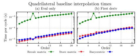
Fig. 4 Baseline interpolation timings for a quadrilateral. (a) Only physical values, (b) Physical and first-derivative values.
