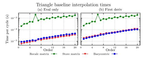
Fig. 6 Baseline interpolation timings for a triangle: (a) Only physical values and (b) Physical and first-derivative values.
