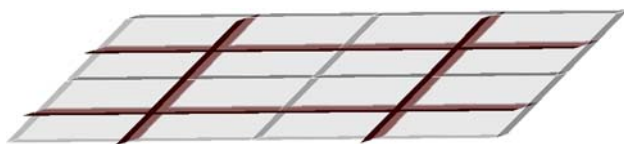
Fig. 10 As sheet intersections deviate from orthogonality, the skew of the mesh increases
